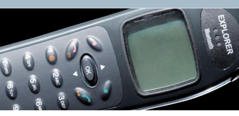
The EXPLORER Bluetooth handset is a cordless telephone handset designed to connect wirelessly via Bluetooth to satellite terminals such as the Thrane & Thrane EXPLORERs. That way you can talk on the phone with anybody anywhere in the world — without strings.
