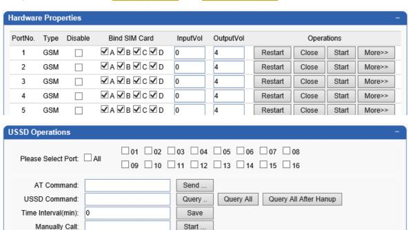
The gateway hardware modules are controlled by "AT Command", and the SIM can get extend service by sending USSD Command from SIM operator. Checking frequency is supported to limit in "Time Interval". And calls can happen directly in "Manually Call" to callee number typed, it's easy to check SIMs inside if they are working, no need to take out SIM and insert it to mobile phone anymore.
