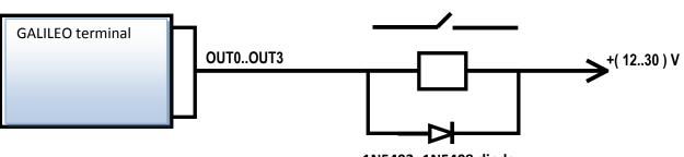
1N5402..1N5408 diode or a similar one for 3 A direct current and reverse voltage at least 200 V
