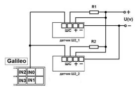
Connection order of 2  $\amalg$ 2 sensors through resistors to one of DAI of the terminal.
