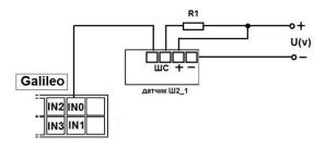
To connect 2 III2 sensors to one of DAI use divisor on two resistors. Calculation principle is realized on voltage level change at sensors triggering.
