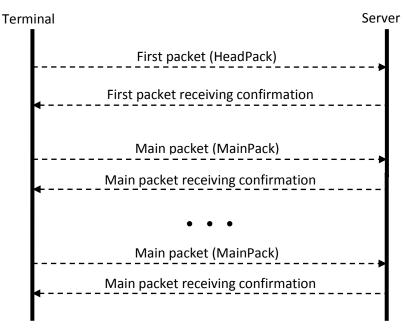
After establishing device-server connection the device sends head pack and then main packs with the data. Each pack needs conformation from the server; if confirmation is not received the terminal sends the pack once again.
