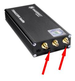
The second SIM-card should be inserted in a similar way.
