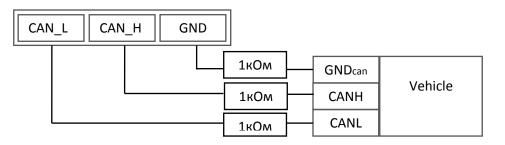
Use the first variant of connection to plug the device into the diagnostic outlet. *The second variant is recommended* to connect the device directly to the CAN bus of a vehicle.
