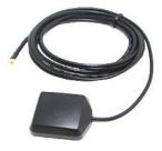
If GLONASS antenna is mounted correctly, your coordinates will be found in 1.5 minutes. To be sure see that the green LED indicator is on. (*See' LED indicators'*).
