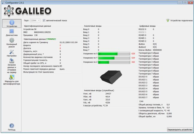
If there is a PIN code in the Terminal, the program will request it to access the settings. At wrong code entering the terminal will disconnect from the computer, reset, connect to the Configurator again and wait for the right code enter.
