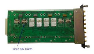
Figure 2-2-1 Push in the GSM user board
