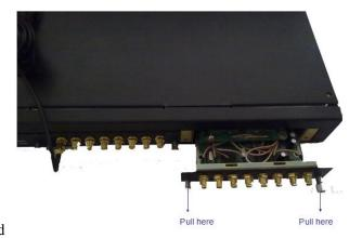
Figure 2-2-1 Pull out the GSM user board
