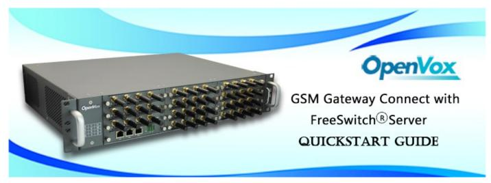
This document applies to OpenVox VS-GW2120 Series GSM Gateway. There are 3 RJ45 Network ports, ETH1/ETH2/ETH3. If you choose ETH1, you can access Board 1 . If you choose ETH2/ETH3, you can access different Boards with different IP addresses.
