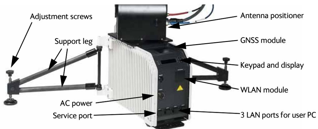
Figure 2-5: Electronics enclosure and support legs
