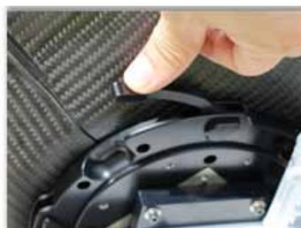
Figure 3-5: Center hub with four latches for the 4 panels
