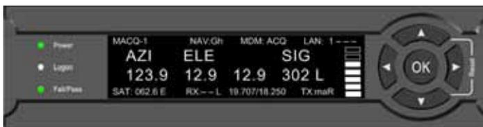
Figure 5-4: Azimuth adjustment, fine tuning
