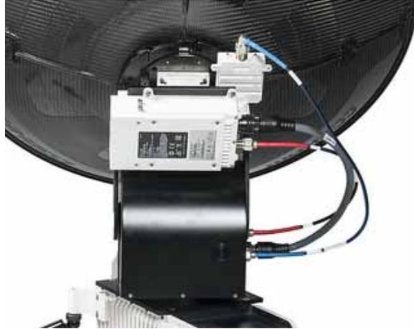
Figure 3-6: Tx, Rx RF and BUC cables
