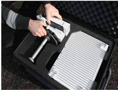
Do not grab the RF assembly by the feed horn. The RF feed's subreflector can be easily damaged.
