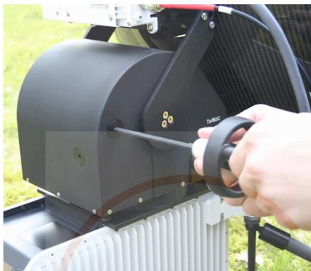
Figure 5-2: Hand crank for manual pointing
