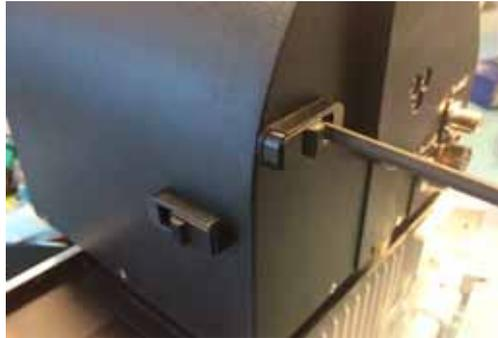
Figure 3-10: Insertion point for the hand crank
