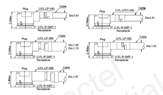
Figure 38: Space Factor of Mated Connector (Unit: mm)
