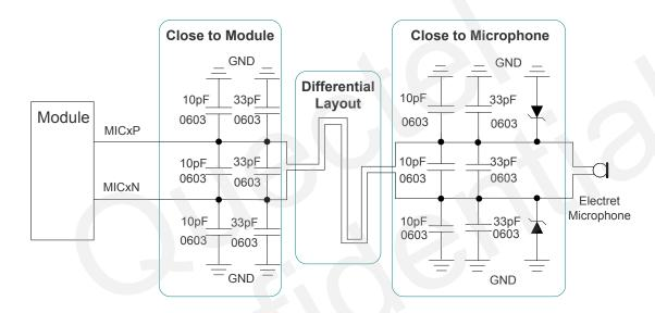
Figure 21: Microphone Reference Design for AIN1&AIN2
