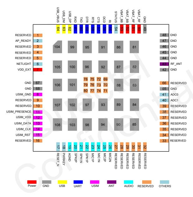
Figure 2: Pin Assignment (Top View)
