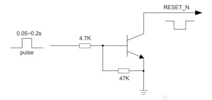
Figure 12: Reference Circuit of RESET\_N
