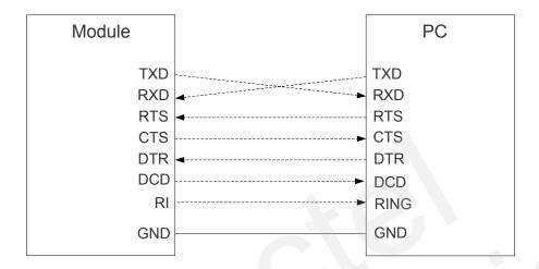
Figure 14: Connection of Full Functional UART Port
