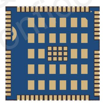
Figure 44: Bottom View of the Module
