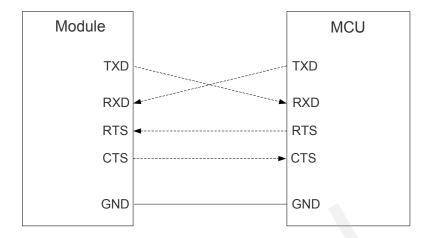
Figure 16: Connection of UART Port with Hardware Flow Control
