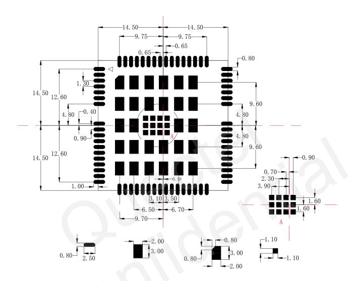
Figure 42: Recommended Footprint (Top View)
