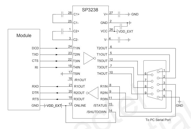
Figure 19: RS232 Level Shift Circuit
