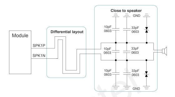
Figure 22: Reference Design for AOUT1
