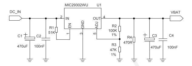
Figure 7: Reference Circuit of Power Supply
