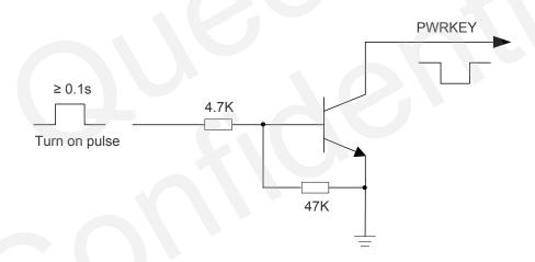
Figure 8: Turn on the Module by Driving Circuit
