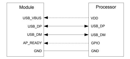
Figure 4: USB Application with Suspend Function
