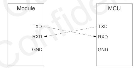
**Figure 15: Connection of Two Lines UART Port**
