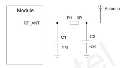
Figure 35: Reference Circuit of Antenna Interface
