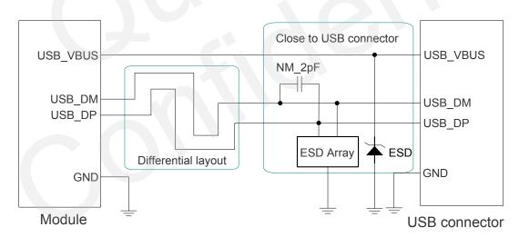
Figure 31: Reference Circuit of USB Application
