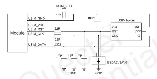
Figure 28: Reference Circuit of the 6 Pin USIM Card
