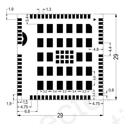
Figure 40: UC15 Bottom Dimensions (Bottom View)
