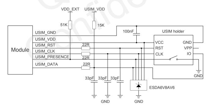
Figure 27: Reference Circuit of the 8 Pin USIM Card
