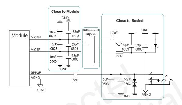
Figure 26: Reference Design for an Earphone
