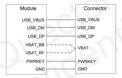
Figure 32: Test Points of Firmware Upgrade
