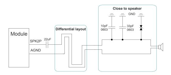
Figure 24: Reference Design for AOUT2
