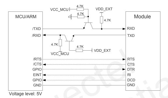
Figure 18: 5V Level Match Circuit
