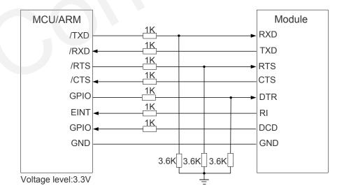
Figure 17: 3.3V Level Match Circuit
