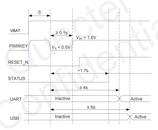
Figure 10: Timing of Turning on Module
