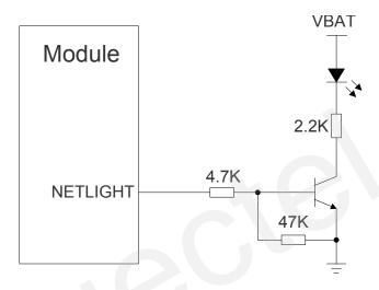
Figure 33: Reference Circuit of the Network Indicator
