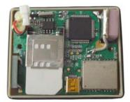
**5.1.4** Connecting the battery as below, and close the back cover by tighten the screws.
