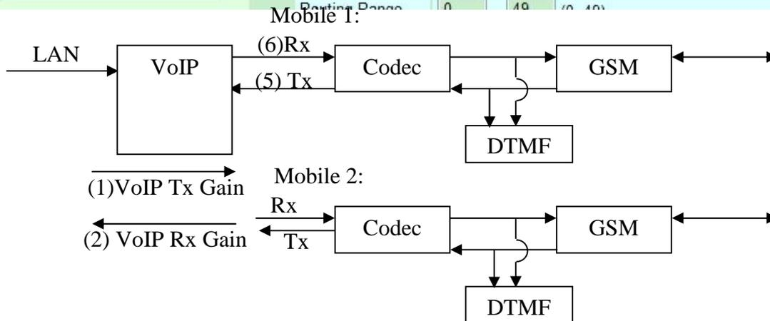
(1) VoIP Tx Gain: To adjust the volume of LAN side.
