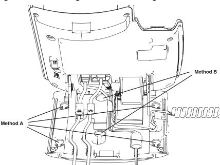
Figure 6: Cable routing tracks and mounting holes
