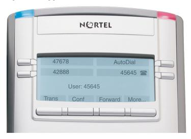
Figure 10 shows an IP Phone 1140E logged in as a Remote phone to an IP Phone 1120E Office phone. Fewer display lines are available on the IP Phone 1120E, so the display provides less information.
