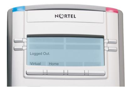
When activated for Virtual Office by a Remote telephone, your Office telephone is *logged out* and no longer operational. If this is the case when you return to your office, you can disconnect the remote login and regain control of your Office phone. If you do not disconnect the remote login, your Virtual Office session expires after a fixed period of time, determined by your system administrator.
