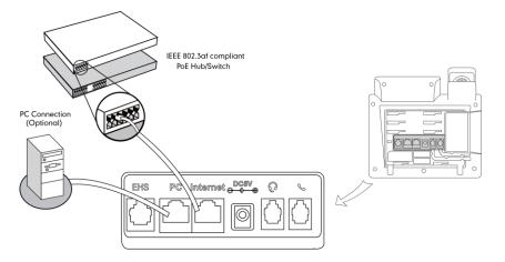
**Note** If in-line power switch/hub is provided, you don't need to connect the phone to the power adapter. Make sure the switch/hub is PoE-compliant.
