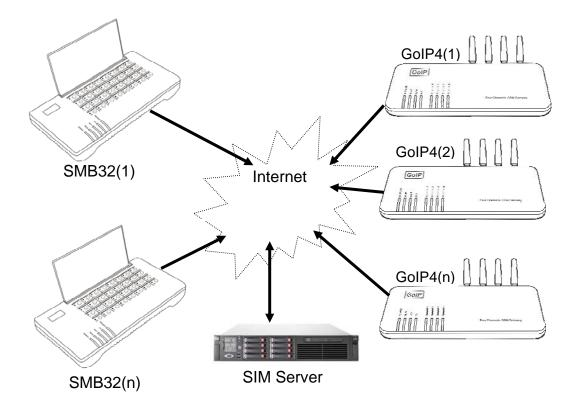
More than 10,000 SIM cards can be collectively scheduled and managed via the SIM Server. The planned tasks are allocated by the SIM Server (SIM Bank mode: client mode)
