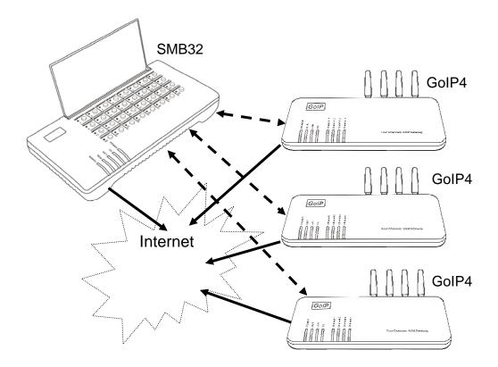
As shown in the above figure, several GoIP devices (up to 32 ways) can be connected to the SMB32 through Internet. The SIM cards installed with the devices are all integrated to the SMB32 to be controlled and scheduled by the latter. (SIM Bank mode: server mode)
