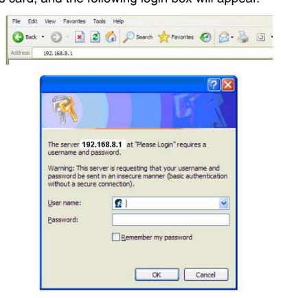
Enter the user name and password to log on the configuration interface (the initial user name and password are both "admin"). \* If you change the setting, remember to press "save the change" to save the configuration.
