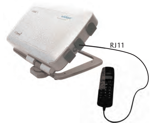
FIGURE 4.1.1-1: Figure showing the connection of the Corded Analog Handset to the RJ-11 Interface of SABRE™ I.
