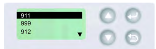
FIGURE 4.1.4-2: LCD showing the list of emergency numbers that are available for selection after user selects the Emergency Call icon from the Menu.
