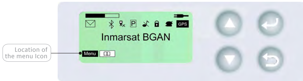
FIGURE 3.6.5-1: Figure showing the location of the “Menu” icon on the LCD display.
