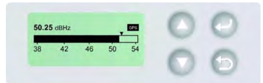
FIGURE 3.6.3-5: LCD display indicating the Signal Strength Bar
