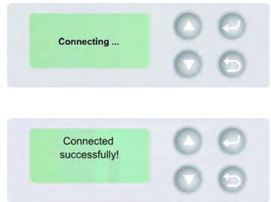
FIGURE 4.5.2.3-1: LCD Display of SABRE™ I showing that a successful IP connection has been established after network parameter configuration.
